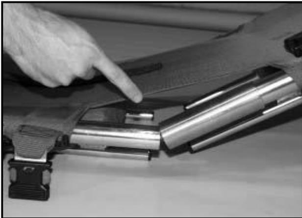
2. Raise the foot section and align the plastic guide pins of the couplers. Lower the foot section into place. Depress pins, and slide both couplers forward into the locked position. Caution: Ensure that both locking pins have fully engaged the sliding coupler.
