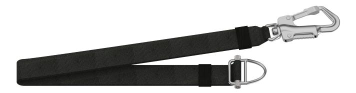
The #467 Restraint Tether is constructed from MIL-SPEC webbing with a high strength stainless steel adjuster on one end and a #513 Safety hook on the opposite end. It has a 3000 lb. breaking load and 600 lb. Working Load Limit. NSN 4240-01-647-9166
